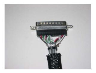
11. Carefully position each connector body into a DB-25 hood, as shown below. If you are using an polyester or fiberglass braided cover, then slide this cover under the clamp on the hood.
